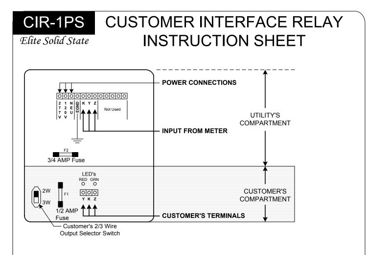
MOUNTING POSITION - The CIR-1PS may be mounted in any position.
