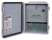
the fusing contained within the customer compartment. The lower compartment, the customer compartment, contains a terminal strip, fusing, status indication LEDs, and a switch that allows the customer to choose either a 2-Wire or 3-Wire output. With the switch in the two-wire mode, each relay contact closure is approximately 100 milliseconds long and occurs each time the 3-Wire input changes state. The red LED will only light each time there is a contact closure.
