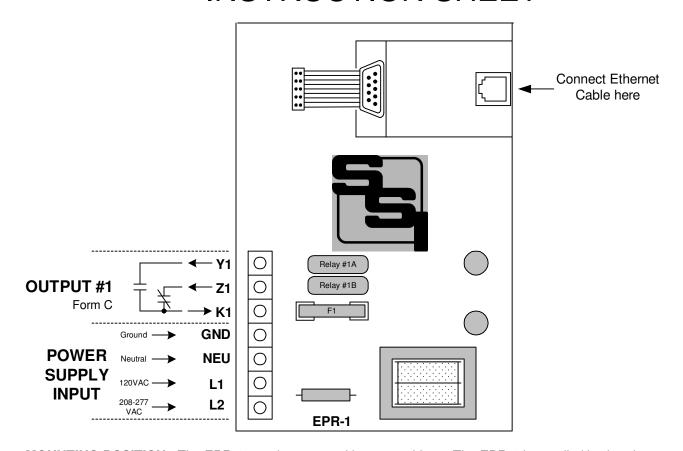
**MOUNTING POSITION** - The EPR-1 may be mounted in any position. The EPR-1 is supplied in chassis form, meaning the PCB assemby is mounted on a chassis for mounted in another metering or instrumentation enclosure.
