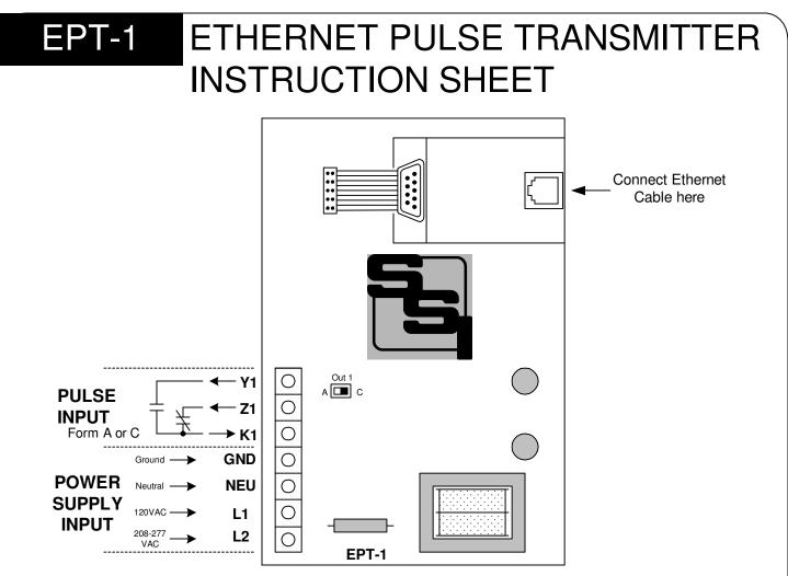
**MOUNTING POSITION -** The EPT-1 may be mounted in any position. The EPT-1 is supplied in chassis form, meaning the PCB assemby is mounted on a chassis for mounted in another metering or instrumentation enclosure.
