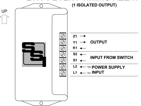
**MOUNTING POSITION -** Because the ETR-1 contains a mercury-wetted relay, it must be mounted in a vertical position to operate correctly.
