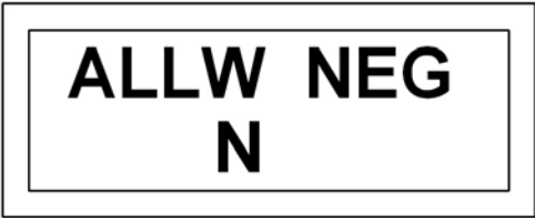
DO NOT ALLOW NEGATIVE ACCUMULATOR DISPLAY
