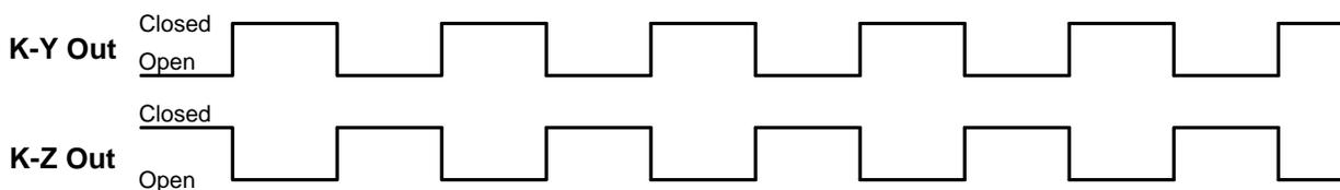
In the Fixed output mode, shown in Figure 2 below, an output pulse (K-Y closure only) is a fixed width (T1) each time the output is triggered. The pulse width (closure time) is determined by the setting of the W command. This mode is best for energy (kWh) counting systems but is generally not the best for systems doing demand control where pulses are timed to derive instantaneous kW demand. The K-Z output is not used in the normal/fixed mode. However, it is used in the Signed mode. See Page 6.
