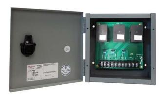
The APU-3 is for 120 VAC applications. The application for the APU-3 is metering configurations where two or more services are provided to the customer, but meter potentials are only on one service. To insure that the meter is always energized and measuring energy use, the APU-3 switches from the primary source to one of 3 auxiliary source if the primary source is lost.
