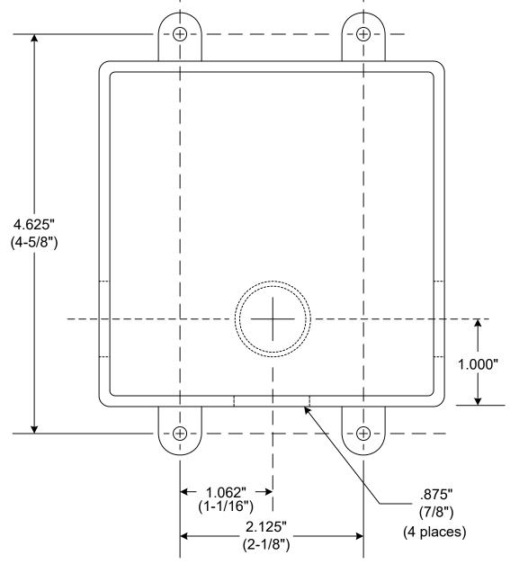
Enclosure has four knockouts for 1/2" conduit connections.
