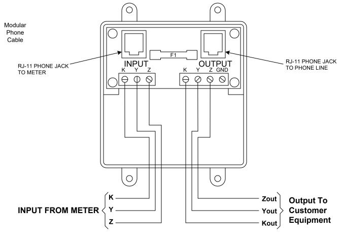
**MOUNTING POSITION** - The CID-4 can be mounted in any position. Use the knockouts on the back and sides to nipple the CID-4 onto the meter enclosure.
