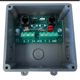
modem and the incoming phone line, while supplying additional surge protection against transient voltage that may affect the inner wirings of the site. Connections to an electric meter's modem to the telephone line are compact, simple and easy.
