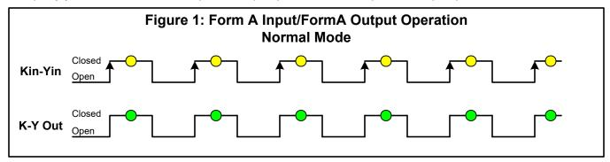
Mode 2 - Form A In/Form A Out with fixed Output Pulse Width: In this Fixed Width mode, the Form A output(s) follow the Form A input, but close for the selected pulse width duration.
