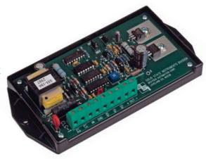
scaling of interpretation of a value of a pulse. The output can be configured so that a K-Y closure will result in either 4mA or 20mA. Once set, the K-Z closure becomes the opposite milliamp output. In this way, a KYZ pulse output can be configured to interface directly to a process control system or other instrumentation with a 4-20mA input.
