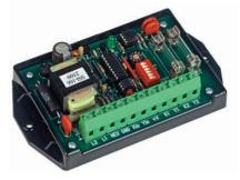
or with a set of needle nose pliers. The DPR-1 counts the input pulses for division only when a correct and valid sequence of pulses occur. Bright yellow and green LED lamps indicate the input and output status of the system at all times thus allowing a rapid visual check-out of the system's performance without requiring any additional test equipment.
