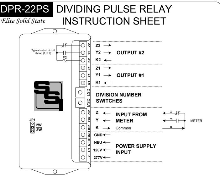
**MOUNTING POSITION** - The DPR-22PS may be mounted in any position.
