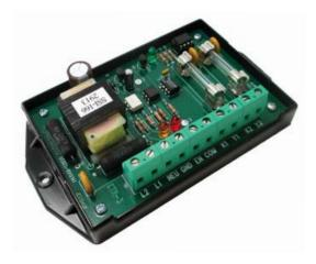
pulse duty cycle is 50/50. Upon receiving each pulse from the meter, the ETR-3's circuitry counts the incoming pulses and keeps in a running count in the count register. When the count register reaches the pre-determined count then a pulse is outputted the next count cycle begins.
