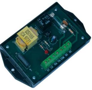
The LCR-1 has a built-in low voltage transformer isolated power supply and may be used with meters having mechanical output contacts (relays), or high or low voltage semiconductor outputs.
