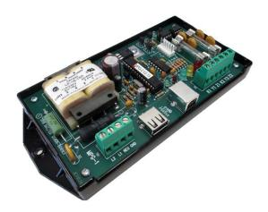
The MPG-1C features a USB input to host the Zigbee radio module "dongle" (included) and two KYZ pulse outputs. As the MPG-1 receives periodic data from utility's meter, the data is read and interpreted to obtain the current demand information. The accumulated energy is computed and pulses are outputted according to a selected pulse value.
