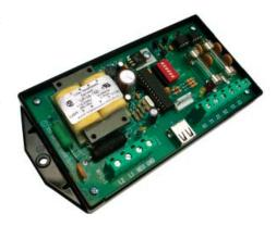
The MPG-1 features a USB input to host the Zigbee radio module "dongle" (sold separately) and two KYZ pulse outputs. As the MPG-1 receives streaming data from utility's meter, the data is read and parsed to obtain the current demand information. The accumulated energy is computed and pulses are outputted according to a selected pulse value.
