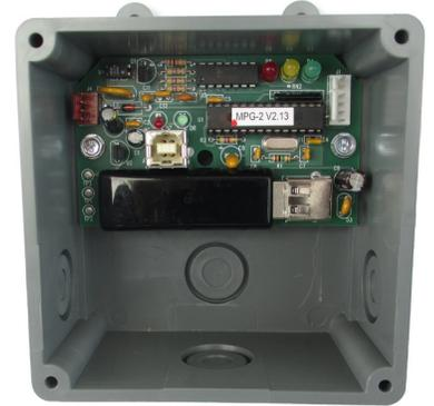
The MPG-2ES features a USB input to host the Zigbee radio module “dongle” (included) and one KY pulse output. As the MPG-2ES receives periodic usage data from the utility’s meter, the data is read and interpreted to obtain the current demand information. The accumulated energy is computed and pulses are outputted according to a selected pulse value.
