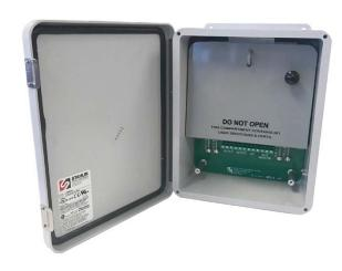
The MPG-2 features a USB input to host the Zigbee radio module "dongle" (included) and two KYZ pulse outputs. As the MPG-2 receives periodic usage data from utility's meter, the data is read and interpreted to obtain the current demand information. The accumulated energy is computed and pulses are outputted according to a selected pulse value.
