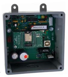
The low-cost "bare bones" MPG-3ES features integral Zigbee radio module and one KY (Form A, 2-Wire) pulse output. The MPG-3ES has a low-voltage AC or DC power supply input for use with other control products having a low voltage source already available. No line voltage source is required.
