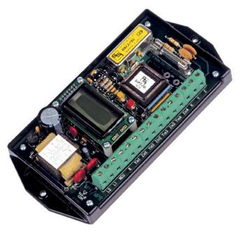
viewed on a LCD display at any time without disturbing the operation of the unit. Typical applications include sub-metering, check metering, and customer-side-of-the-meter applications where a readout of totalized energy from multiple meters is desired. The input pulse signal from the sending device to the MPR-4 is by four sets of "Y" & "Z" leads with a common "K" lead.
