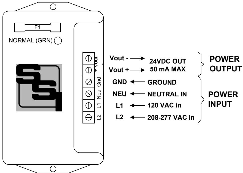
**GENERAL** - The MPS-1-24 is a power supply for KYZ Pulse Metering. It is designed to provide a "wetting" or sense voltage to the "K" terminal of a KYZ pulse initiator or KYZ isolation dry contact output. This sense voltage is switched on and off as the KY and KZ terminals are closed to source this voltage to another "downstream" device which does not supply its own wetting voltage.
