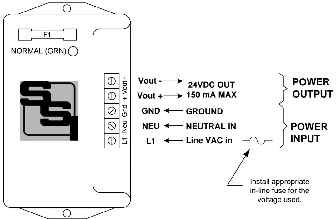
**GENERAL** - The MPS-2-24 is a power supply for KYZ Pulse Metering. It is designed to provide a "wetting" or sense voltage to the "K" terminal of a KYZ pulse initiator or an isolated dry-contact output. This sense voltage is switched on and off as the KY and KZ terminals are closed to source this voltage to another "downstream" device which does not supply its own wetting voltage.
