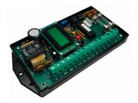
The MPT-2C's output module may be operated in 1-channel or 2-channel mode. In 1-channel mode, the MPT-2C operates with a single KYZ output channel. In 2-channel mode, the MPT-2C operates with two independent KY output channels, each having a unique output value. In both configurations, there are two physical outputs on each channel, eliminating the need for an additional "splitting" or pulse duplicating relay.
