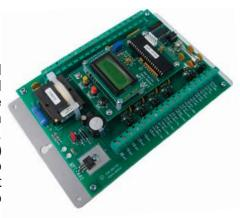
The MPT-440's output module may be operated in 1-channel or 2-channel mode. In 1-channel mode, the MPT-440 operates with a single KYZ output channel. In 2-channel mode, the MPT-440 operates with two independent KY output channels, each having a unique output value. In both configurations, there are two physical outputs on each channel, eliminating the need for an additional "splitting" or pulse duplicating relay.
