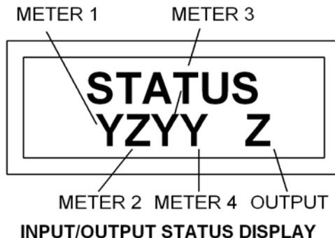
The “Z” displayed as an output status shows that the contacts between “K” and “Z” on the output are closed or “made up”. The “K” to “Y” output contacts are open. **PRESS THE ORANGE KEY TO GO TO NEXT DISPLAY.**
