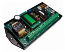
The MPT-4C's output module may be operated in 1-channel or 2-channel mode. In 1-channel mode, the MPT-4C operates with a single KYZ output channel. In 2-channel mode, the MPT-4C operates with two independent KY output channels, each having a unique output value. In both configurations, there are two physical outputs on each channel, eliminating the need for an additional "splitting" or pulse duplicating relay.
