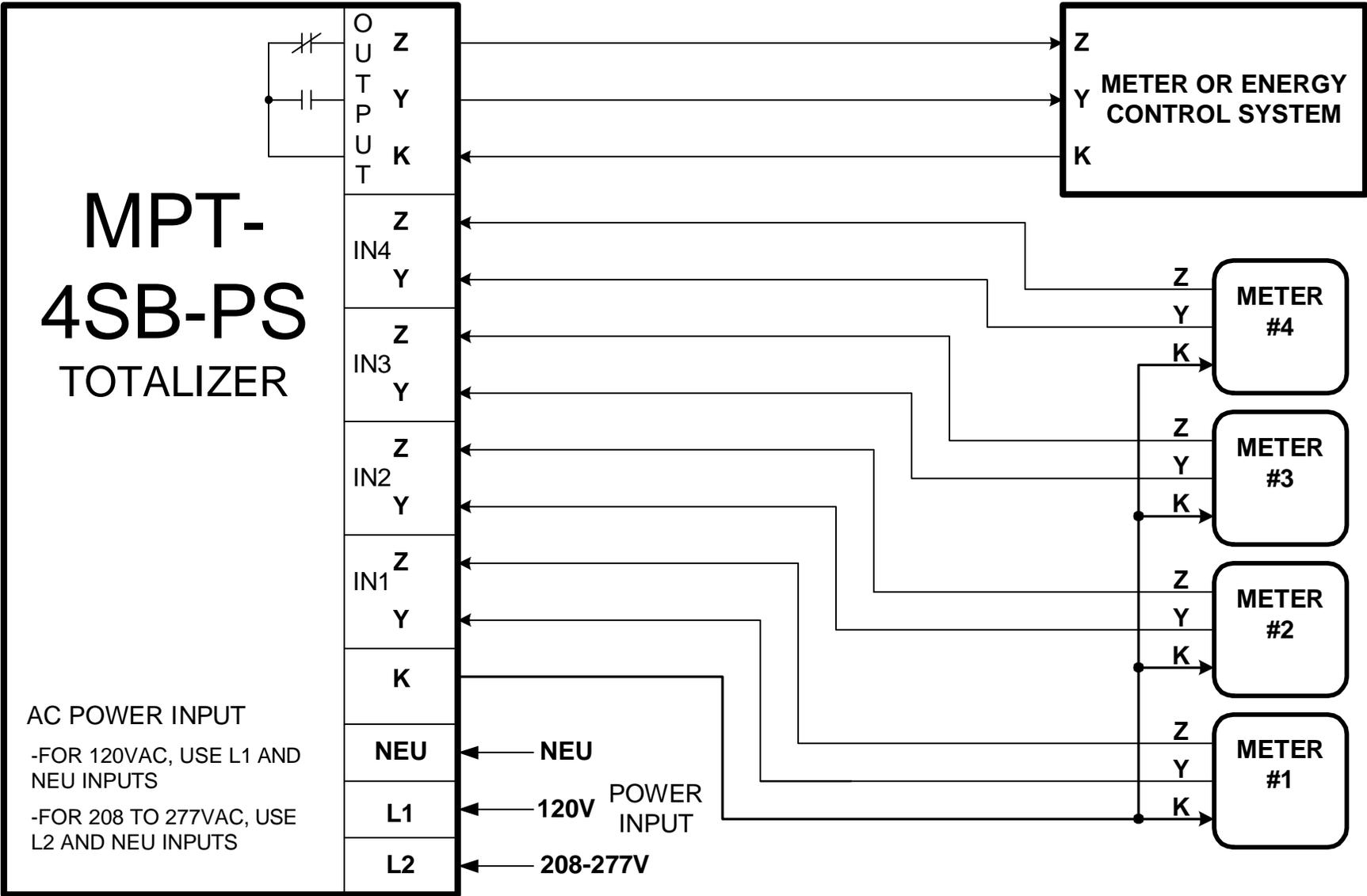
NOTE: A Sense Voltage of +13VDC is applied to the meters via the "Y" or "Z" leads from the MPT-4SB-PS. The "K" lead is the common return.
