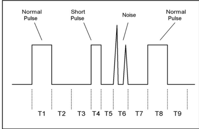
power systems are less than one cycle long, we recommend that the minimum setting be 30 milliseconds. This still allows a pulse input rate to the MPT-8B of 33 pulses per second, a rate much higher than usually experienced. The absolute minimum setting that the MPT-8B will accept is 10 milliseconds. The maximum time is 250 milliseconds. Entry is in 10 millisecond increments. The entry process is the same as that used with the meter input values.
