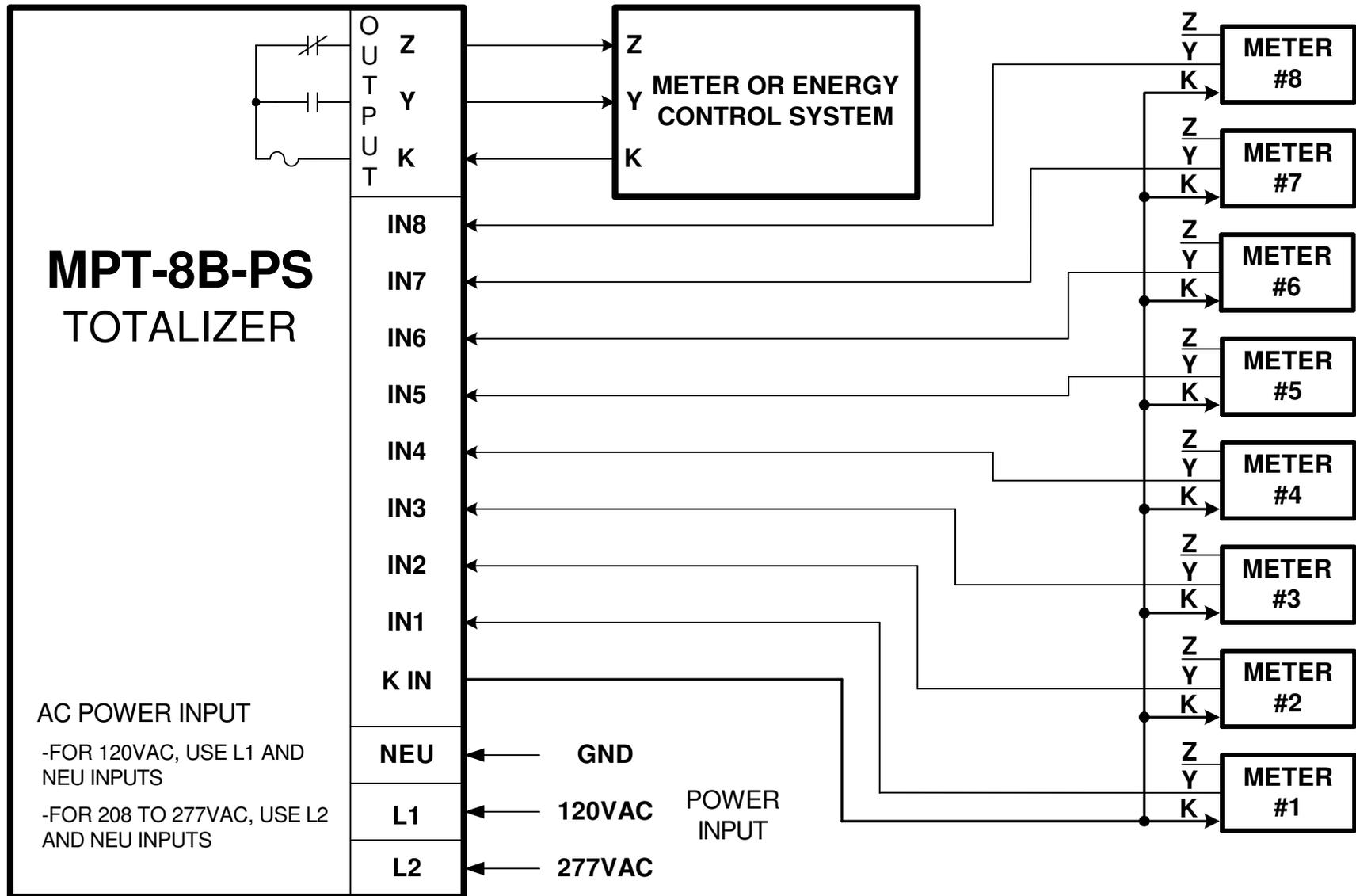
NOTE: A Sense Voltage of +13VDC is applied to the meters via the "Y" or "Z" leads from the MPT-8B-PS. The "K" lead is the common return.
