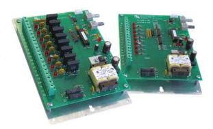
The OPL-4C system makes it possible to quickly implement a 4-channel optical pulse link with minimal effort. The system includes the power supply, wetting voltage, isolation relay and terminal block connectors making it possible to have a multichannel optical link up and running in minutes. The OPL-4C utilizes standard "ST" twist lock connectors and makes connections reliable, quick and easy. The multimode fiber optic cable is not included.
