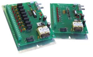
The OPL-8C system makes it possible to quickly implement an 8-channel optical pulse link with minimal effort. The system includes the power supply, wetting voltage, isolation relay and terminal block connectors making it possible to have a multichannel optical link up and running in minutes. The OPL-8C utilizes standard "ST" twist lock connectors and makes connections reliable, quick and easy. The multimode fiber optic cable is not included.
