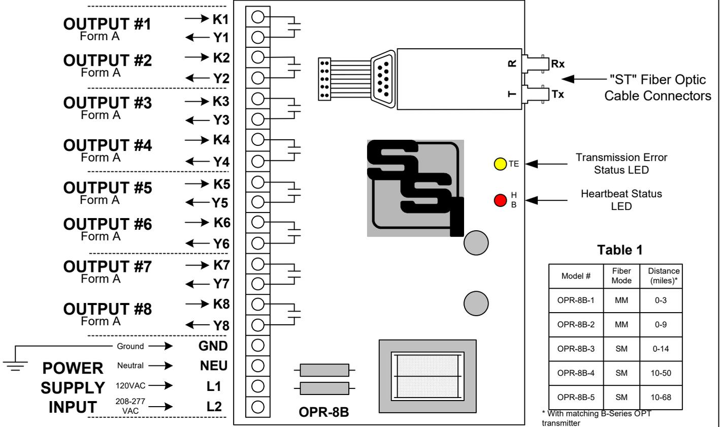
**MOUNTING POSITION** - The OPR-8B may be mounted in any position.
