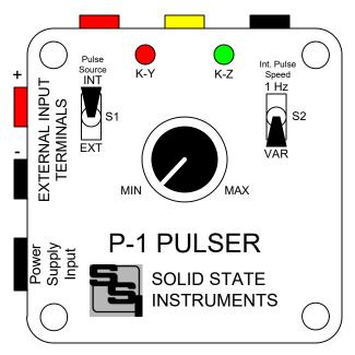
**FUNCTION -** The P-1 is a handy pulse generator designed to test pulse receiving equipment by simulating the pulse output of an electric meter. Form A (2-Wire) with K and Y terminals, or Form C (3-Wire) with K, Y and Z terminals.
