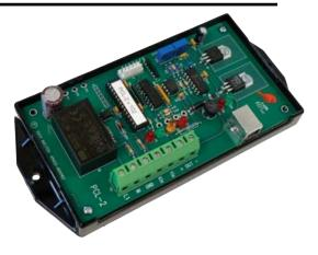
receiving each pulse from the meter, the PCL-2's microcontroller calculates the instantaneous rate of usage based on the pulse rate and value, and updates the output to a current level between 4mA and 20mA. For example, suppose you have the full-scale output of the PCL-2 configured for 500kW. If a current demand of 250kW is calculated, the output would be adjusted to 12mA, the 50% midpoint between 4 and 20mA.
