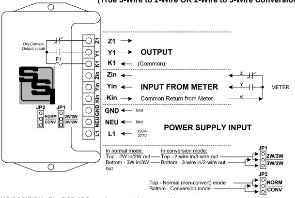
**MOUNTING POSITION** - The PCR-3PS may be mounted in any position.
