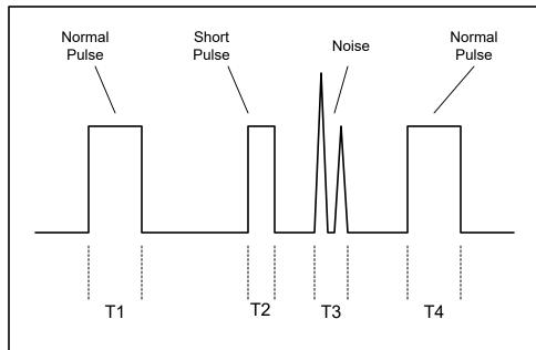
the time the input pulse is present. If the input pulse is present for less than the specified time (in milliseconds) as determined by the position of jumpers JP4 and JP5. it is assumed to be noise. An input equal or longer in duration than the specified time is classified as a valid input and an output will occur. In the illustration to the left.
