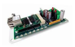
the meter, the PMC-1's microcontroller converts the pulse to the kWh value and adds it to the energy use register. The instantaneous, average and peak demand (kW) are also captured and available in three separate registers for each channel. Average and Peak Demands are based on a 15 minute demand interval.
