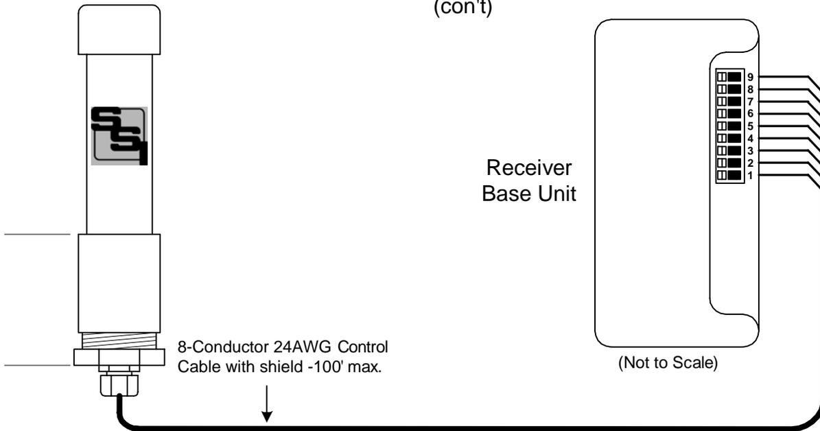
**POWER INPUT** - The PRR-900 receives its power supply from the PRR-2 Receiver Base unit.
