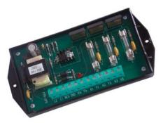
outputs (K & Y). Its current loop design will adjust the output voltage to overcome and compensate for the resistance of the wire loop.
