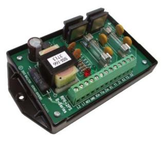
The RPR-2PS relay is designed to filter noise and transients from its input to prevent any false pulses at its output. Bright red and green LED indicators display the system's status at all times thus allowing a rapid visual check of the system's performance without requiring any additional test equipment.
