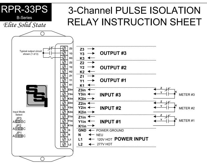
**MOUNTING POSITION** - The RPR-33PS may be mounted in any position.
