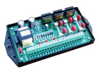
The RPR-33PS relay is designed to filter noise and transients from its input to prevent any false pulses at its output. Bright red and green LED indicators display the system's status at all times thus allowing a rapid visual check of the system's performance without requiring any additional test equipment.
