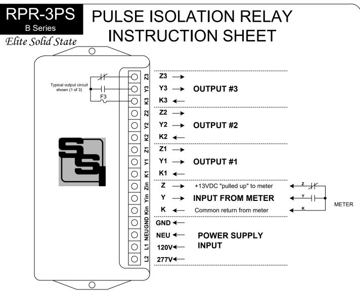
**MOUNTING POSITION** - The RPR-3PS can be mounted in any position.
