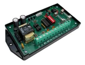
from its "pulled up" state to ground (K) for at least a minimum pulse time. Four input filter times are field-selectable: 50 microseconds, .5, 5 or 20 milliseconds.
