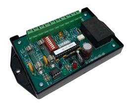
Eight input filter times are field-selectable: 25, 50, 100, 200 or 500 microseconds, or 1, 5 or 20 milliseconds. With the appropriate filtering time, noise that could be counted as pulses is ignored.
