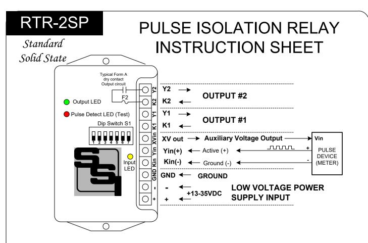
**<u>POWER INPUT</u>** - For a DC power supply of +13VDC to +35VDC, connect the "+" lead to the + terminal. Connect the "-" power supply lead to the - terminal. Connect the electrical system ground to the **GND** terminal. The unit must be grounded for proper operation.
