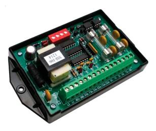
The SPR-22 operates over the standard SSI wide voltage range. The SPR-22 has a built-in low voltage transformer-isolated power supply generating a +13VDC sense voltage. The sense voltage is sent to each electric meter's Y and Z pulse initiator output terminals from the SPR-22's "Y1in"/"Z1in" and "Y2in"/"Z2in" input terminals, returning to the "K1in" and "K2in" terminals, the common return for both meters.
