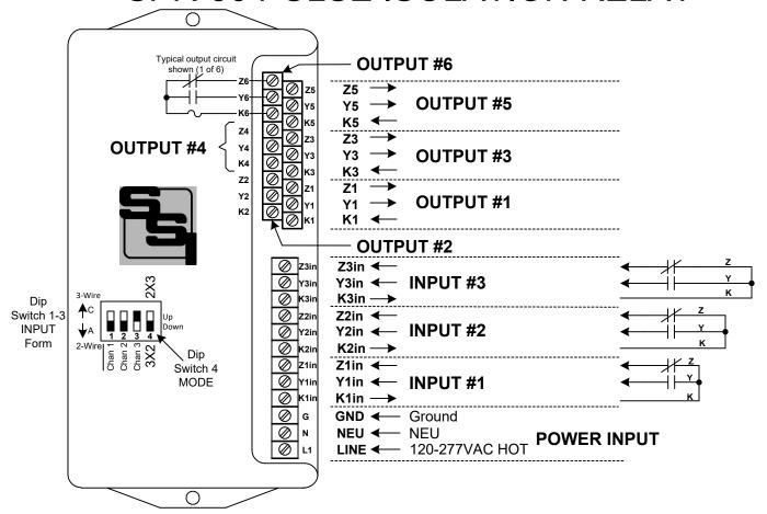
**MOUNTING POSITION** - The SPR-36 may be mounted in <u>any</u> position since it uses solid state relays.
